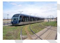
**Light Rail/Diesel Multiple Unit** – A rail transit line that can operate in a variety of settings including dedicated ROW, subway, or mixed on-street traffic. Light rail transit (LRT) usually relies on overhead wires for power and is designed for heavily traveled corridors where the stop needs do not support heavy rail transit, and are typically not compatible with freight rail.
