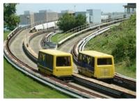
operate on a demand-responsive basis, and work to move travelers directly from origin to destination along a fixed route. Several systems have been built, with the most notable in Morgantown, WV.
