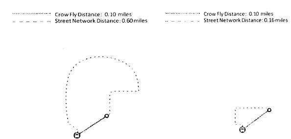
A disconnected street network (shown at left) with long blocks and indirect streets resids in long walking distances and less efficient transit operations. A well-connected street network (shown at right) enables shorter inside direct walking connections and is easier to serve cost effectively with transit.
